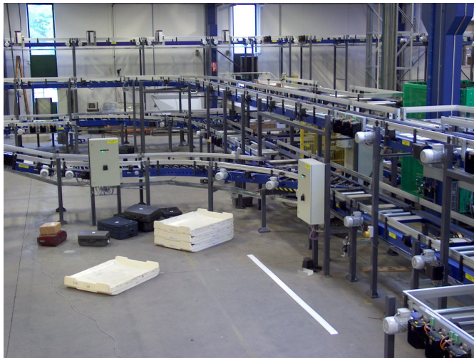
Figure 1.2: BHS hardware setup example
