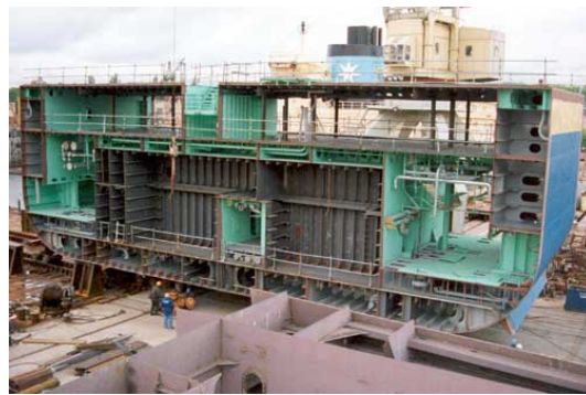
Figure 2.10: A steel section
