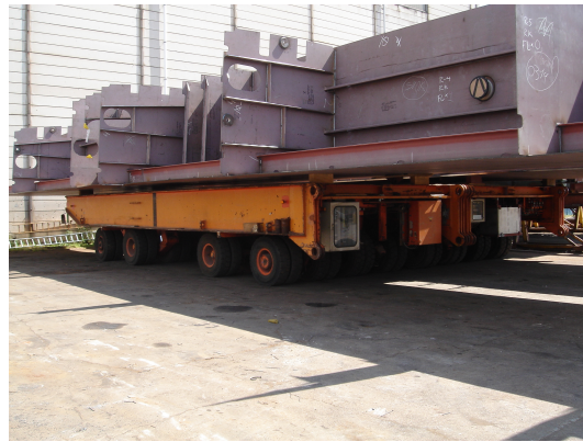
Figure 2.7: KAMAG - transporting a ship block
